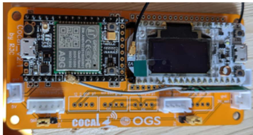
Figure 8. Heltec and A9G board on a PCB designed for COCAL
