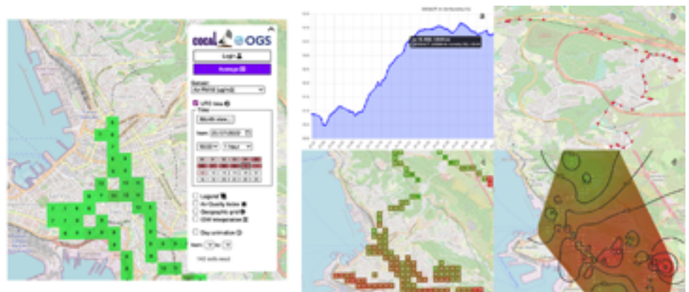
Figure 10. COCAL web-based GUI (left) and near real-time visualizations: a) time series; b) single acquisitions; c) near real-time window averaging; d) interpolation and contour.
