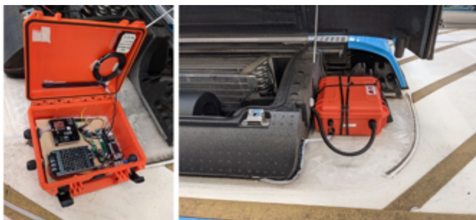
Figure 5. Installing a COCAL box on buses
